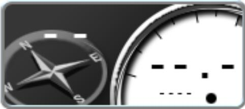
The Heading and Speed widget displays the current GPS heading and vehicle speed as detected by the receiver. Touch and hold this widget to access the GPS Health prompt with additional details on GPS reception.
