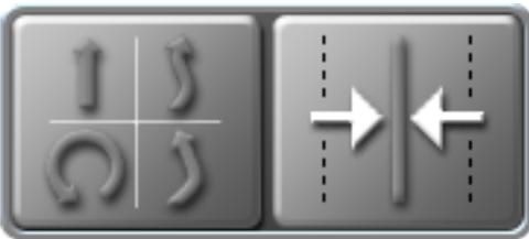
The AB Utilities widget will be necessary to select guidance modes, set AB paths, or to save or load an AB guidance path. Tapping the AB utilities widget will set A and B points for a guidance path (if a guidance path is not set) or access the AB guidance line tools and will provide access the Nudge and Swath prompt.
