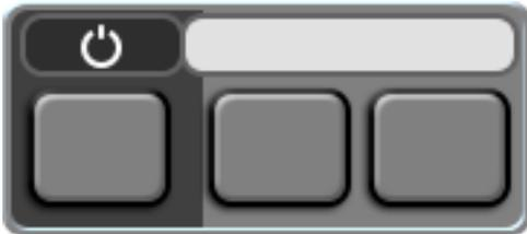
Select the On-Screen Switch box widget to control sections directly on the ROS device during field operations. The on-screen switch box widget will only be available if the on-screen switch box feature has been configured and if a Raven CAN switch box or Switch Pro™ is not detected on the CANbus.
