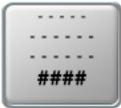
Select the Tally Registers widget to provide a display of total volume, field volume, total area, field area during field operations.
