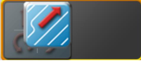
Multi-line coverage is a guidance pattern type in which multiple already created guidance lines are loaded in at the same time. When loaded, the guidance system will attempt to lock onto a nearby line and steer the machine to the detected line until the user attempts to steer to an alternative line.
