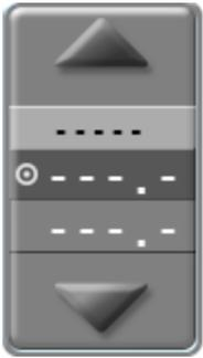
Displays the target and actual application rate for the selected product. This widget allows the user to select the Data Type, Implement, Function or Feature, Data Element, and the product Name. This widget will show status on/off status, volume, and allow the user to increase or decrease flow rate.
