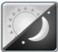
The day/night widget allows the operator to toggle between a day and night display mode during a field operation. Tap the widget to toggle the display mode. Touch and hold the widget to view screen and LED brightness settings for the current mode.
