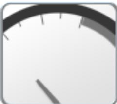
The Vehicle Speed widget displays the current vehicle speed as reported by a speed sense node on the CANbus. The speed displayed using this widget is the speed to which a rate control system will be using for speed compensated rate control systems.
