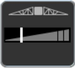
Having the Boom Capacity widget on the run screen provides visibility to the percentage of the boom capacity currently used. This is for information purposes only.
