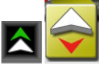
The forward/reverse status indicator shows if the machine is traveling forward or reverse according to the ROS device.
