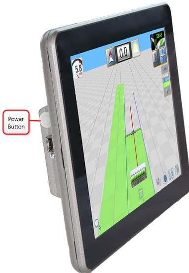
The power button will flash red and then should illuminate green. If the button stays red or does not illuminate, contact a local Raven dealer for additional assistance.
