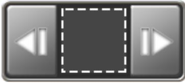
To scroll through various ISO applications, place the ISO Working Set Selector widget on the run screen. This allows the user to have a scroll through all of the items running on the ISObus system. Scroll left or right through the selector to view the available systems on the ISObus system. Press the center of the button to show all available ISO working sets. From the list of available working sets, select a working set to make it active.
