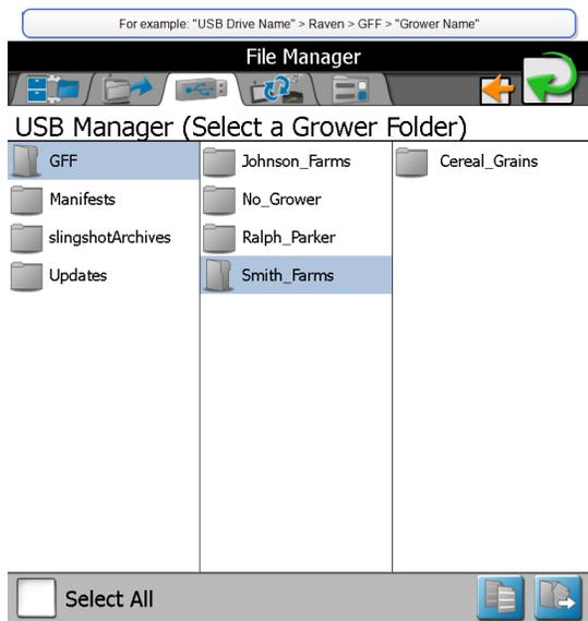
**Note:** When importing the GFF folder structure, only select to the "Grower" folder level of the GFF folder structure. The ROS device will automatically transfer the folder information contained within the grower folder to complete the GFF structure. If farm or field folders are selected, the GFF folder structure will be incorrect when imported to the ROS device.
