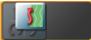
Last Pass is best used for applying around the headlands of a field, in U shaped areas, and circular patterns. Last Pass creates a guidance path based on previous coverage in a field. Every two seconds, last pass searches for a piece of coverage (previously applied area) in order to maintain the guidance path.
