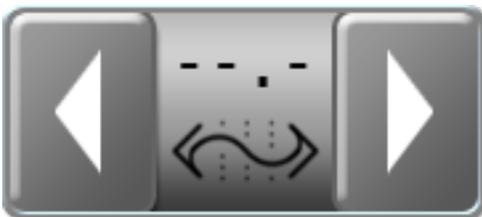
The Nudge Arrow widget offers the same display information as the Nudge Status widget, but provides access to nudge controls directly on the current display view or mode. Select this option to allow the operator to manually adjust the guidance line directly from the guidance display during field operations.
