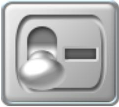
The boom/implement Master Switch widget provides an option for an on-screen master switch to toggle all configured sections on or off. Select this option if a machine switch panel or another switch option is available for toggling boom section status. See "Configure the Master Switch Options" on page 204 for additional assistance with enabling the on-screen master switch feature.
