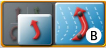
The Fixed Contour pattern is ideal for creating and saving swaths which follow irregular field boundaries, waterways, well heads, etc., or where the ability to skip swaths in an irregular pattern is necessary.
