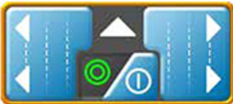
A flip area is primarily used for planting and tilling to create a boundary around the edge of the field or another obstacle that creates a zone that will not be planted. This allows the user to plant the entire field and, when done with everything in the field except for the flip area, go back and plant that area last. See "Create a Flip Area" on page 290 for more information on flip areas and the Flip widget.
