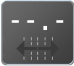
The Nudge Status widget displays the current nudge applied to the displayed guidance line. Touch and hold the Nudge Status widget to access the Nudge and Swath prompt. See "Nudge Features and Tools" on page 269 for more detailed information about operating the Nudge feature.
