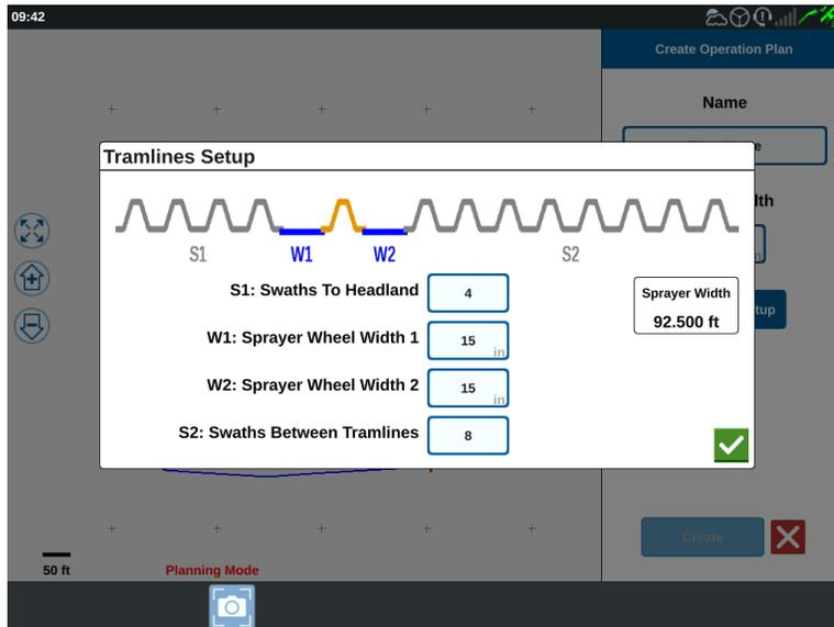
**Note:** Tramlines are spaces between rows that are not planted so future operations in that field (such as spraying) will not drive over rows of crops.
