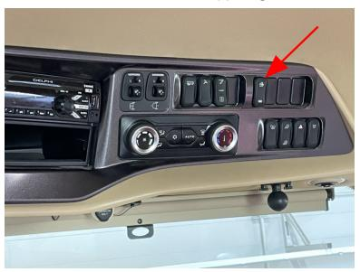
2. Enable the ISOBUS switch by pressing the **Tractor AUTO** icon.
