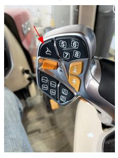
6. Engage propulsion by pressing the button on the back hand side of Multi-Function Handle.
