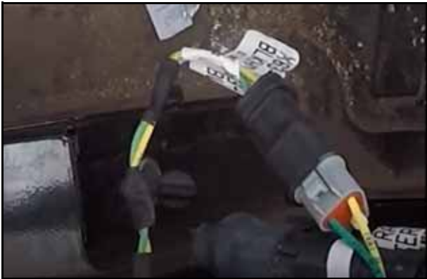
FIGURE 8. X-59 Connected to Raven Vehicle CAN Cable
